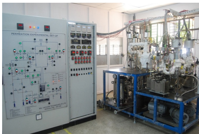
Figure A.2.9.3 Installed setup for hydrogen isotope permeation study
