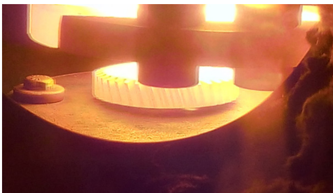
Figure B.1.1 (left) The sample becomes red hot during the heating process. (right) Plasma surrounding the samples during plasma carburizing process
