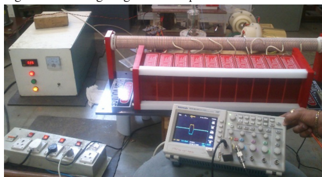
Figure A.3.4.1 The Pulsed Modulator System being developed
