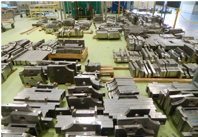
Figure B.2.1 In-Wall Shielding manufactured blocks
